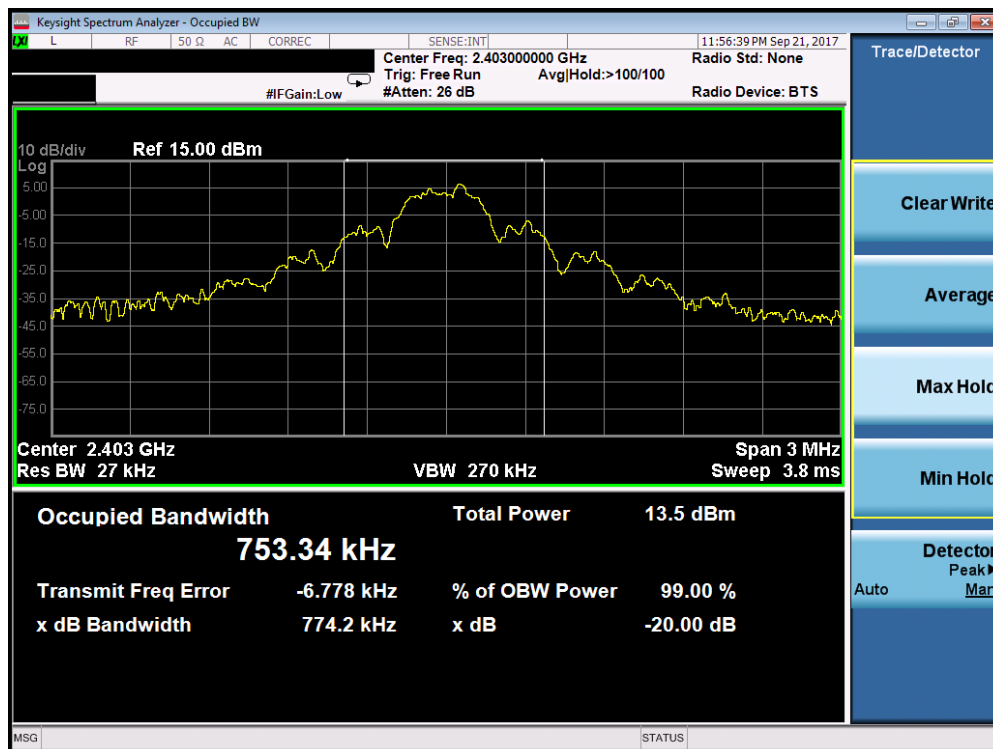
Plot 7-7. 20dB Bandwidth Plot (EX600-WSV1, Ch. 0)
