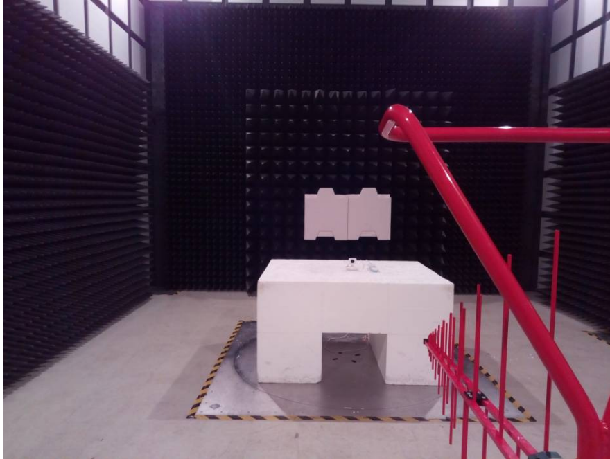
Radiated Emissions Tested View (Below 1GHz, Transmitting)
