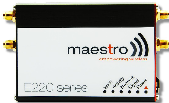
Figure 1: E220 Series: High-speed 3G or LTE router
