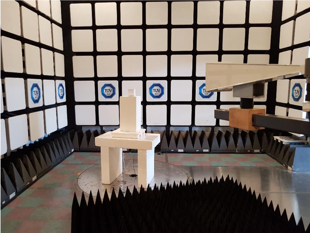
Figure 4 – Radiated Emissions Setup – Photo 3
