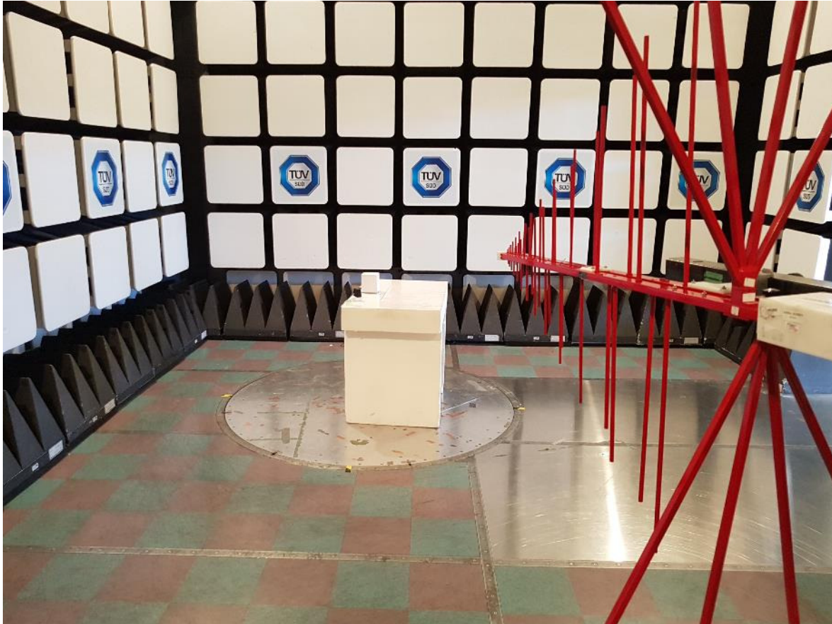
Figure 3 – Radiated Emissions Setup – Photo 2
