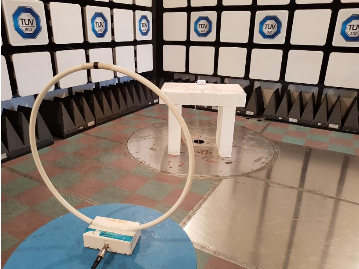
Figure 2 – Radiated Emissions Setup – Photo 1
