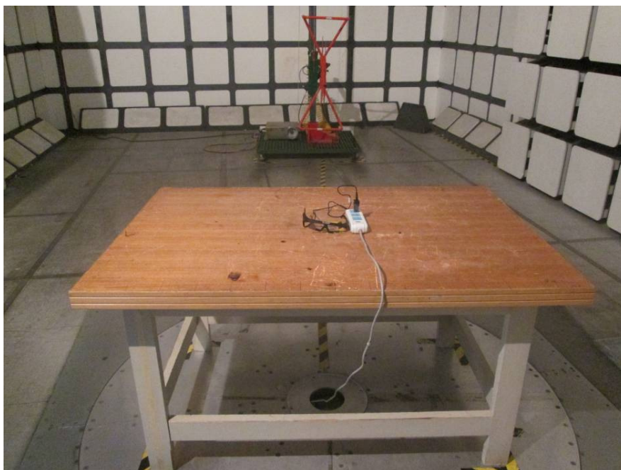
Radiated Emissions View (Below 1 GHz)
