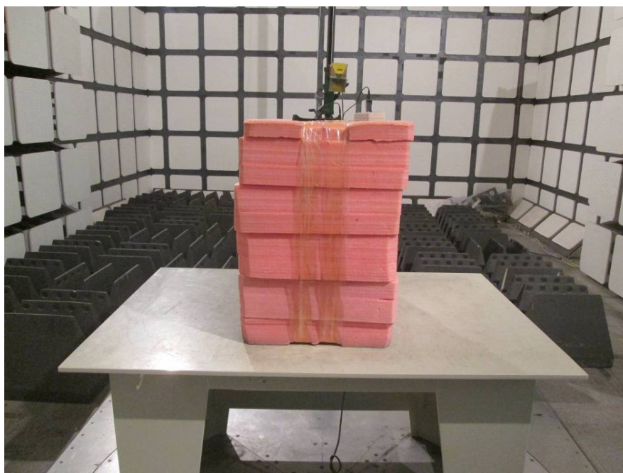
Radiated Emissions View (Above 1 GHz)
