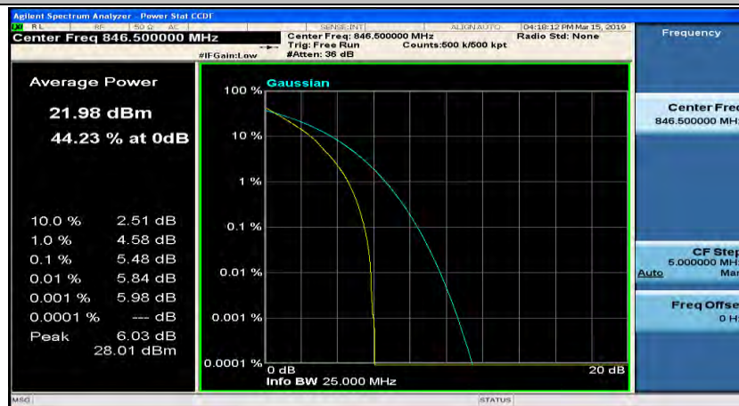
(Channel Bandwidth: 5 MHz)_HCH_QPSK_25RB#0
