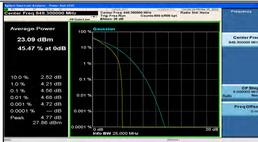
(Channel Bandwidth: 1.4 MHz)_HCH_QPSK_6RB#0
