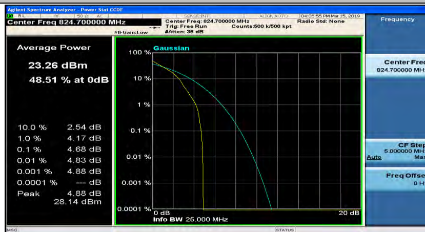
(Channel Bandwidth: 1.4 MHz)_LCH_QPSK_3RB#0
