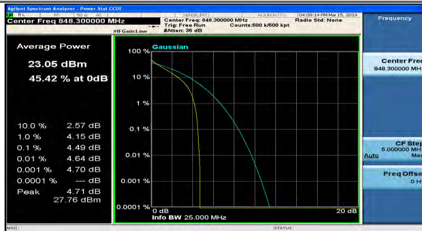
(Channel Bandwidth: 1.4 MHz)_HCH_QPSK_3RB#2
