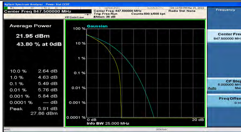
(Channel Bandwidth: 3 MHz)_HCH_QPSK_15RB#0
