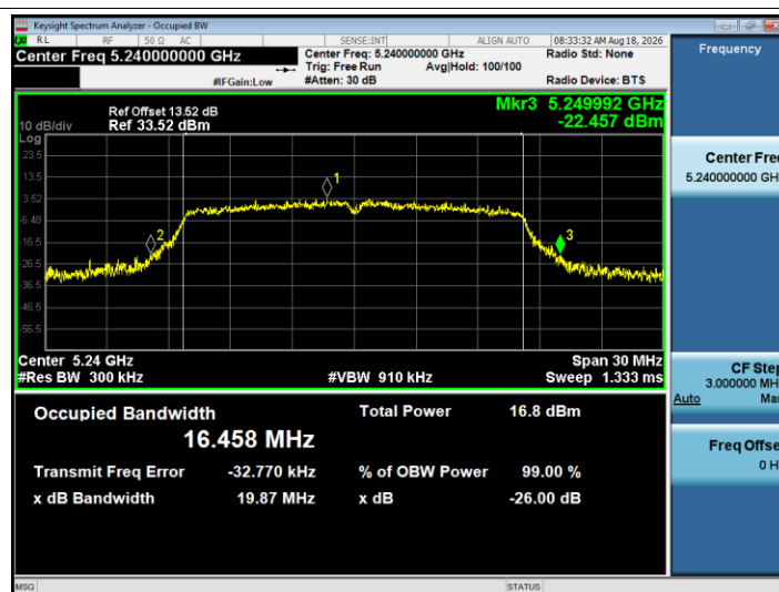
-26dB Bandwidth NVNT a 5240MHz Ant1
