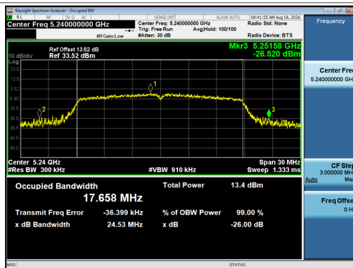
-26dB Bandwidth NVNT n20 5240MHz Ant1
