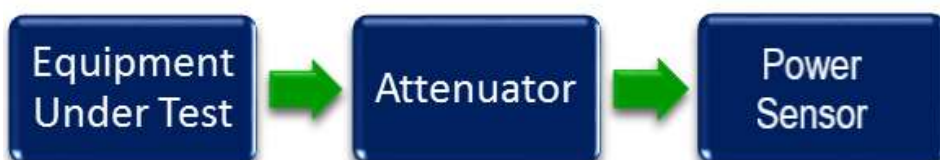
Figure 3. RF Power Test Setup – WIFI
