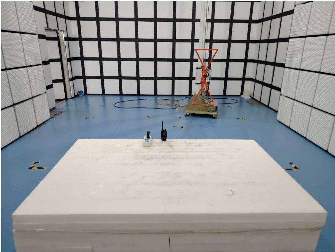
Radiation Emission_Below 1GHz - Back View (Mode 1)
