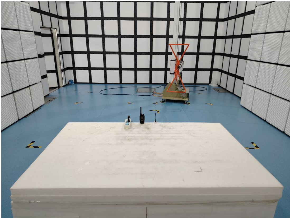
Radiation Emission_Below 1GHz - Back View (Mode 2)
