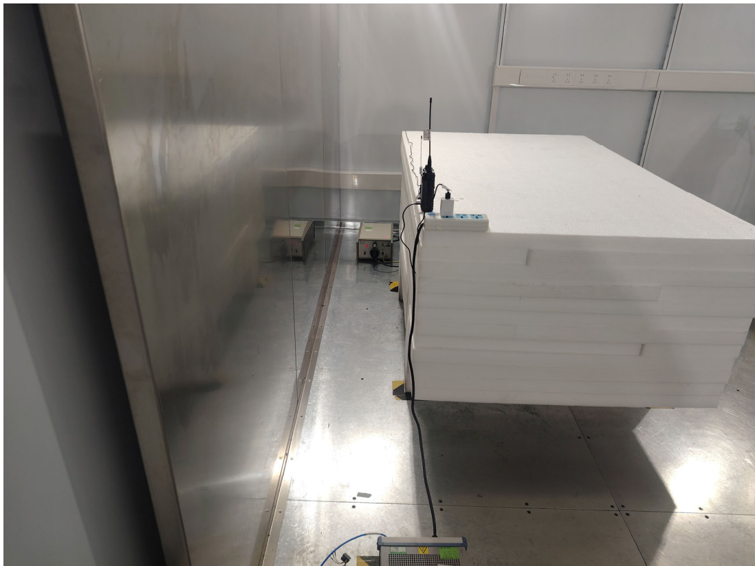
Conducted Emission - Side View
