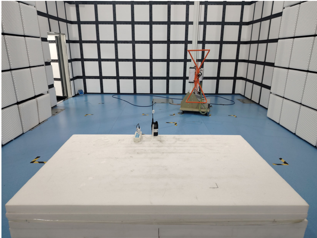
Radiated Emission - Back View (Below 1GHz)
