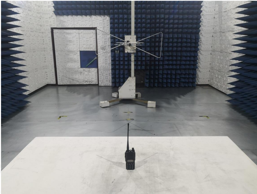
RADIATED EMISSION ABOVE 1G TEST SETUP
