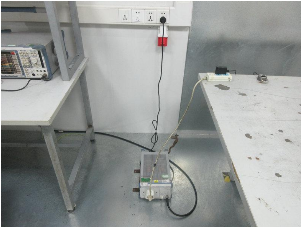
Photo of Power Line Conducted Emission Test
