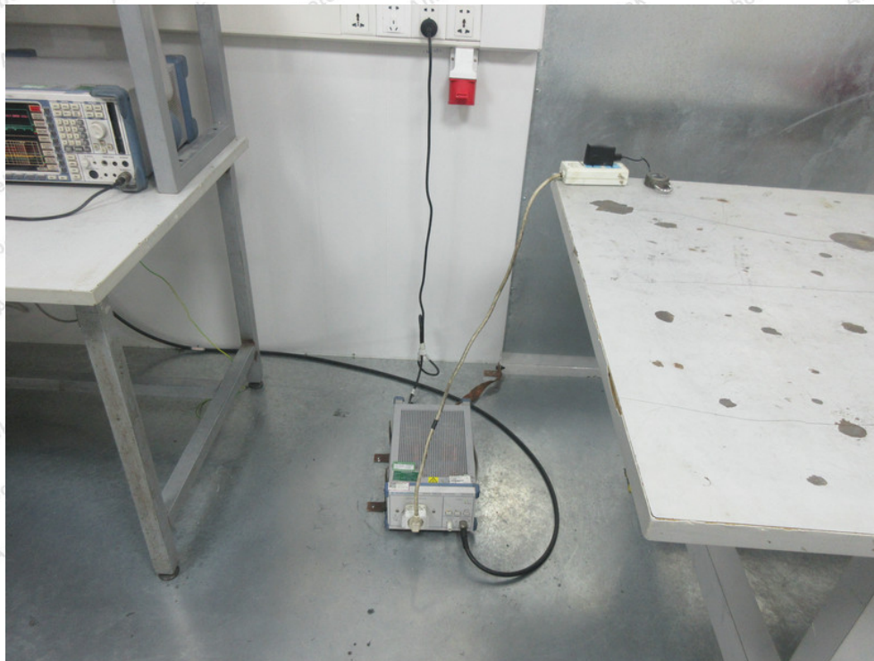
Photo of Power Line Conducted Emission Test
