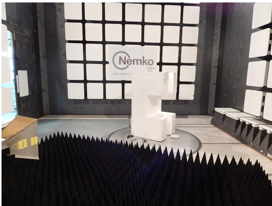
Figure 8.3-15: Radiated spurious (out-of-band) emissions setup photo – 1-18 GHz
