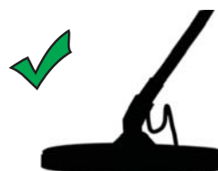
Correct search coil angle
