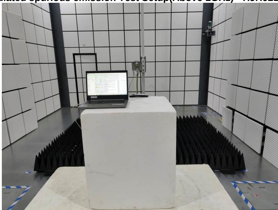
Radiated spurious emission Test Setup(Above 1GHz)-- HJH92B Ble
