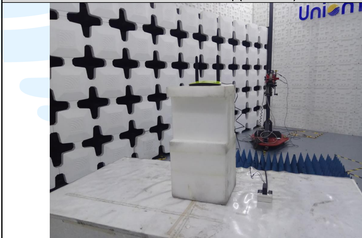
Radiated emission Test Setup (Above 1 GHz)
