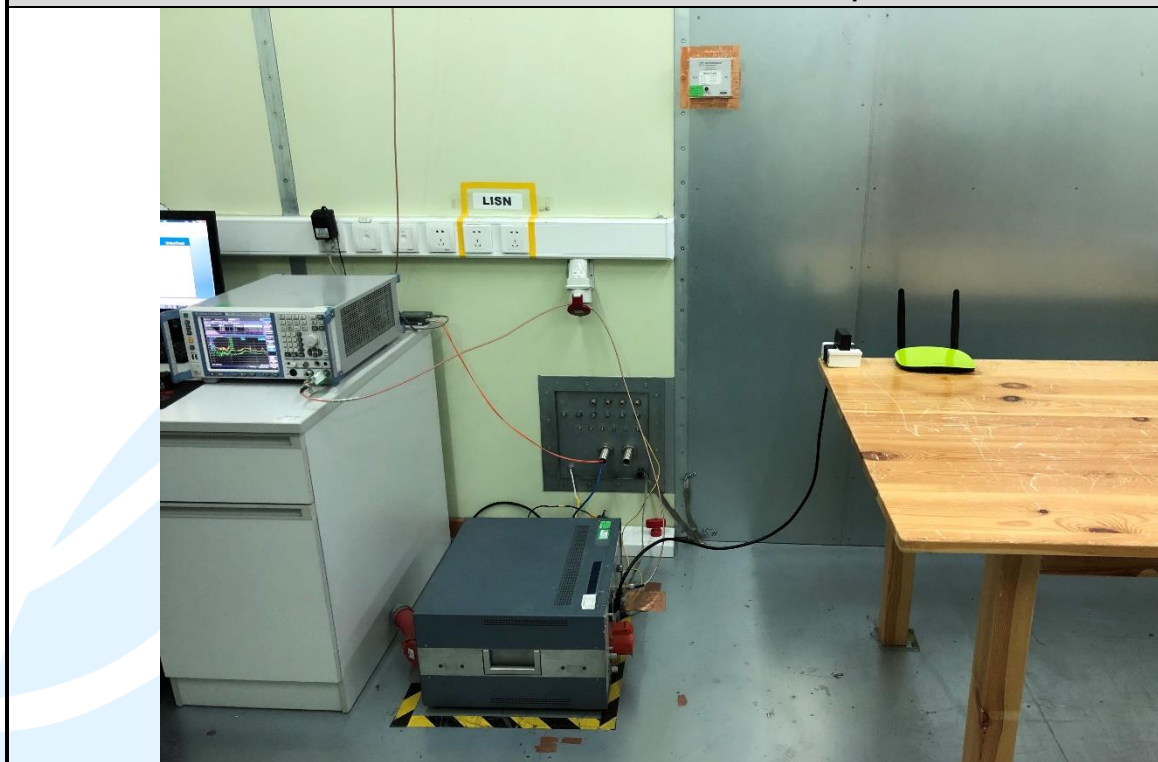
Conducted Emission Test Setup
