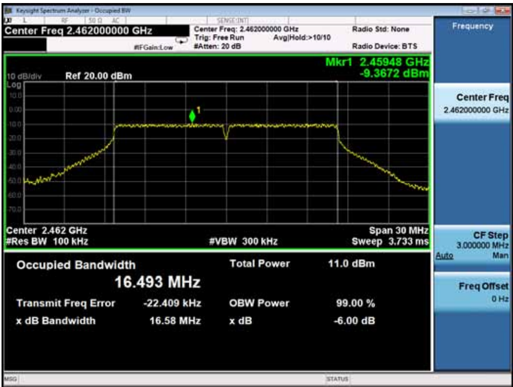
TEST PLOT OF BANDWIDTH FOR HIGH CHANNEL
