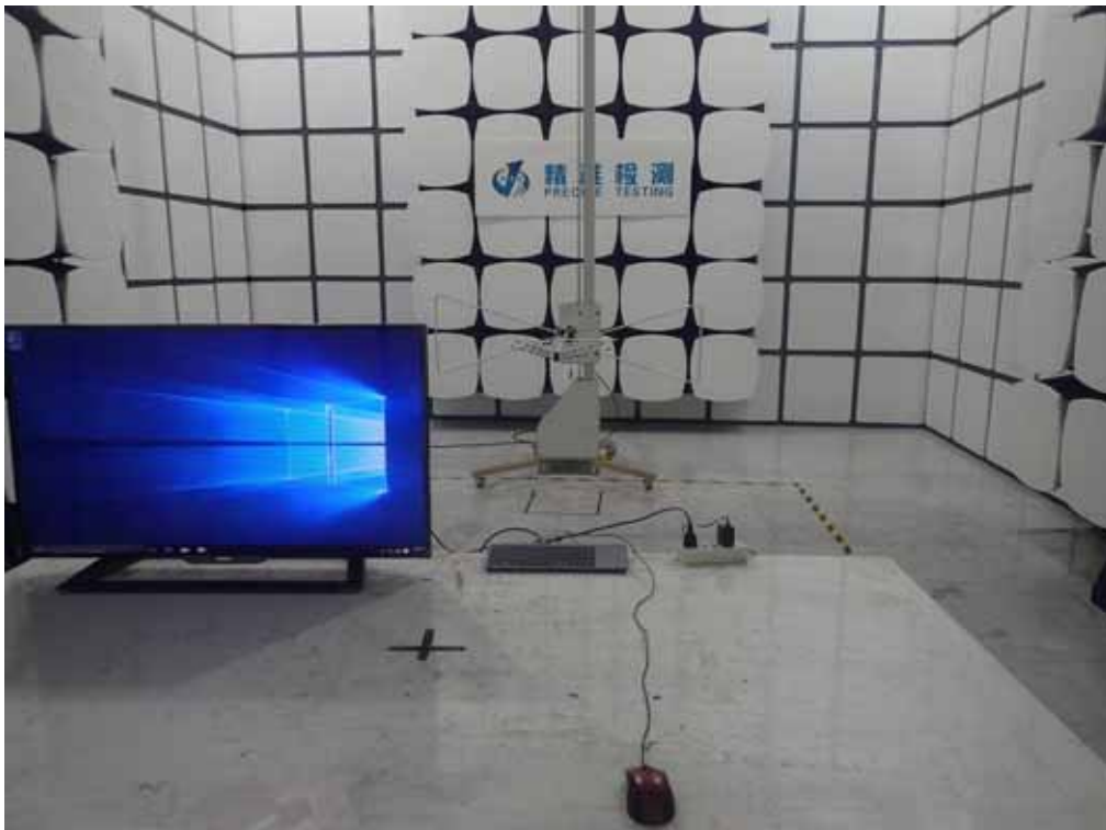
FCC RADIATED EMISSION TEST SETUP BELOW 1GHZ
