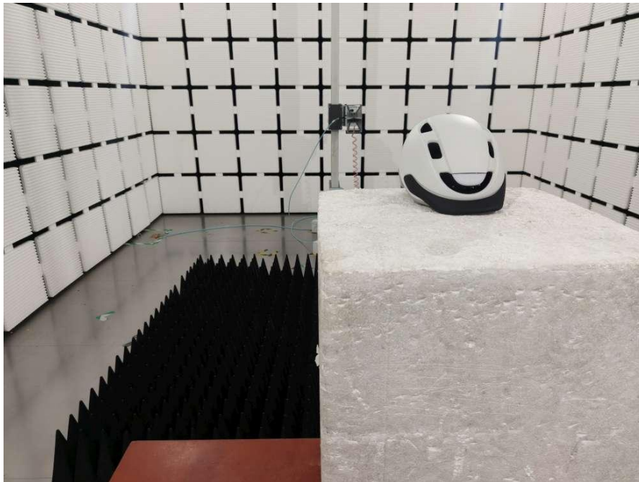
Radiated Emission Test View 2
