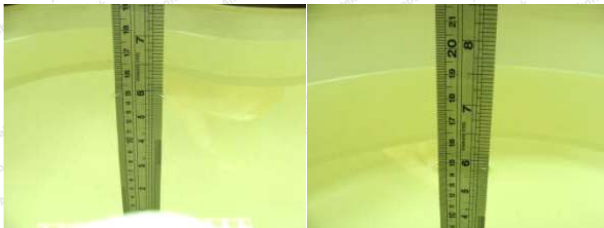
Photo of Liquid Height for Head SAR
