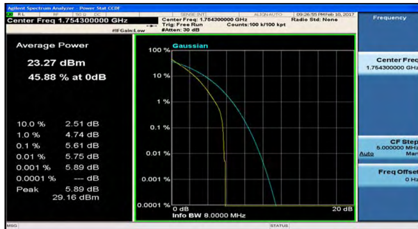
(LTE band 4_Channel Bandwidth: 1.4 MHz)_HCH_QPSK_3RB#2
