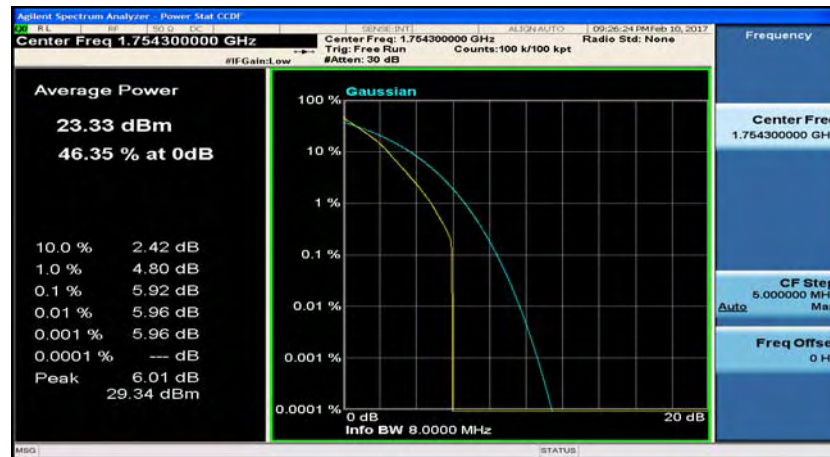
(LTE band 4_Channel Bandwidth: 1.4 MHz)_HCH_QPSK_1RB#3
