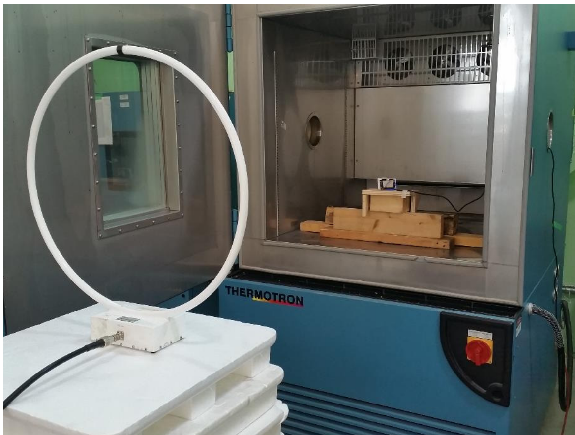
Figure 4 – Carrier Frequency Stability Setup
