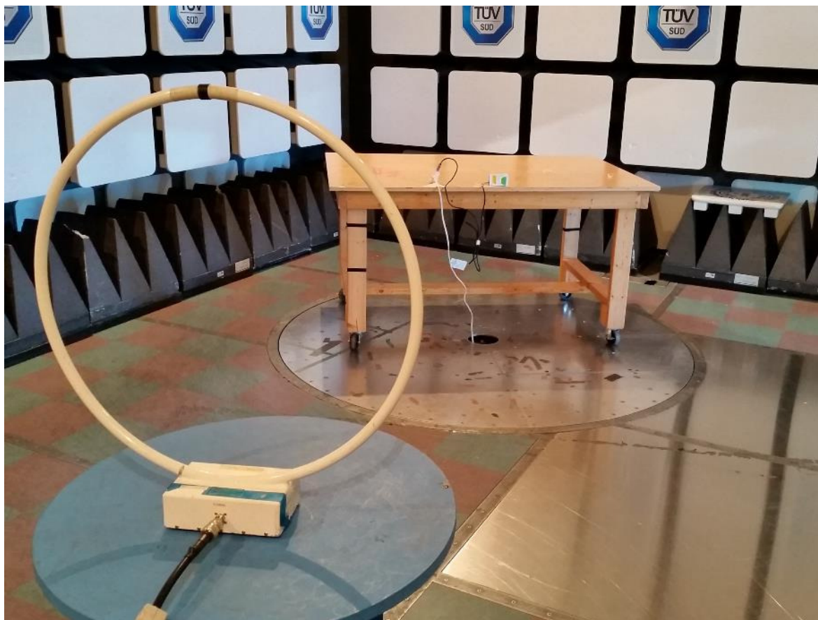
Figure 2 – Radiated Emissions Setup – Photo 1
