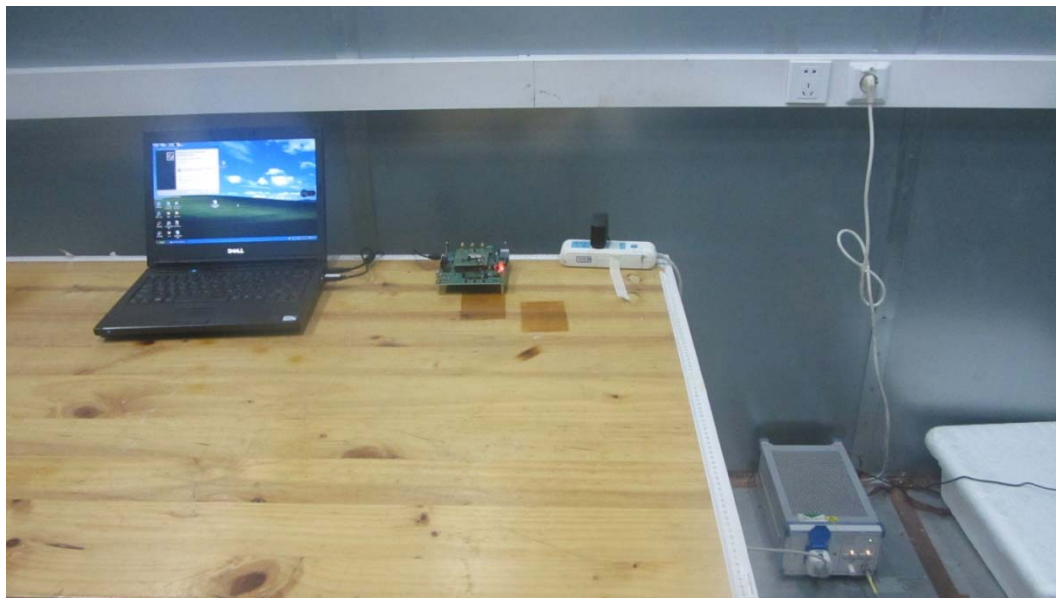
Picture 3 Conducted Emission Test Setup
