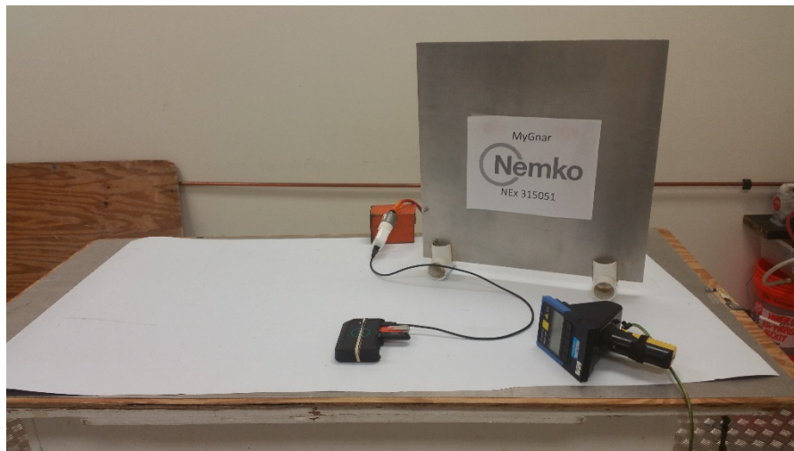
Figure 8.5-3: Clause 9.3 – Electrostatic discharge setup photo
