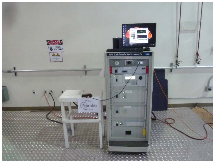
Figure 8.8-1: Clause 9.7 – Voltage dips and interruptions setup photo
