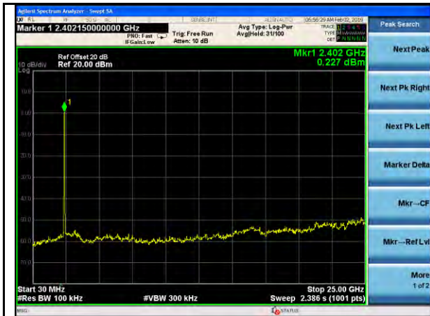
11n 20MHz-Out Of Band Emission-Low
