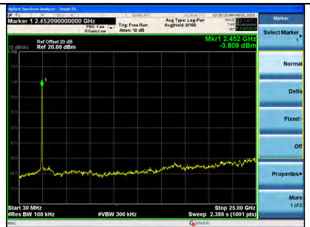
11n 40MHz-Out Of Band Emission-Mid
