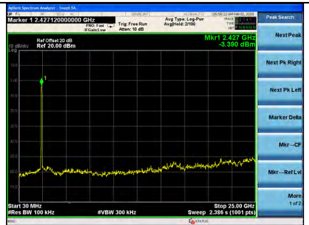
11n 40MHz-Out Of Band Emission-Low
