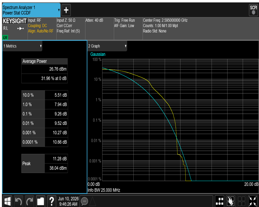
Band41(2535-2655) QAM16 BW=5MHz Channel=40640 RB Size=1 Position=#0
