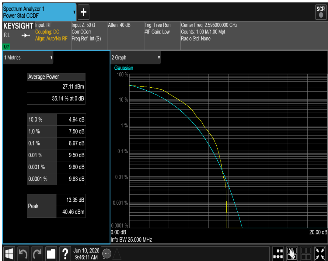
Band41(2535-2655) QPSK BW=15MHz Channel=40640 RB Size=1 Position=#0
