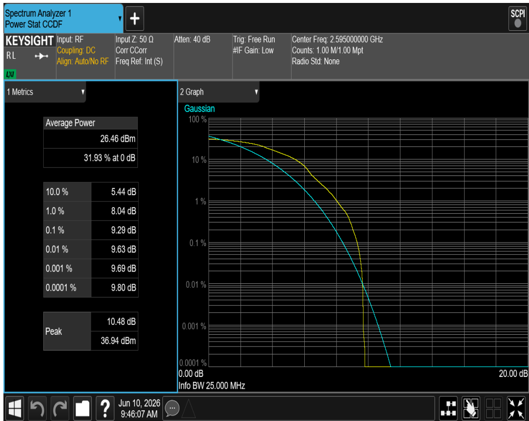
Band41(2535-2655) QPSK BW=10MHz Channel=40640 RB Size=1 Position=#0
