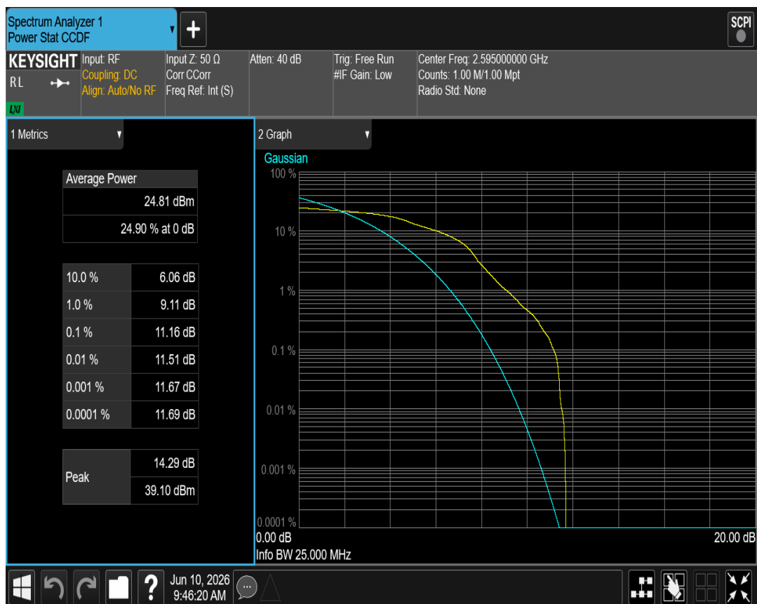
Band41(2535-2655) QAM16 BW=20MHz Channel=40640 RB Size=1 Position=#0
