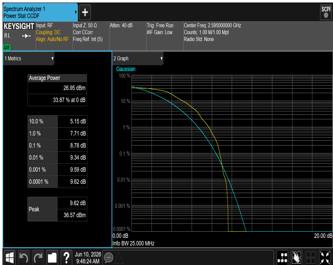
Band41(2535-2655) QPSK BW=5MHz Channel=40640 RB Size=1 Position=#0
