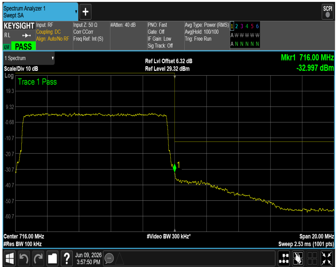
Band17 QPSK BW=5MHz Channel=23755 RB Size=25 Position=#0
