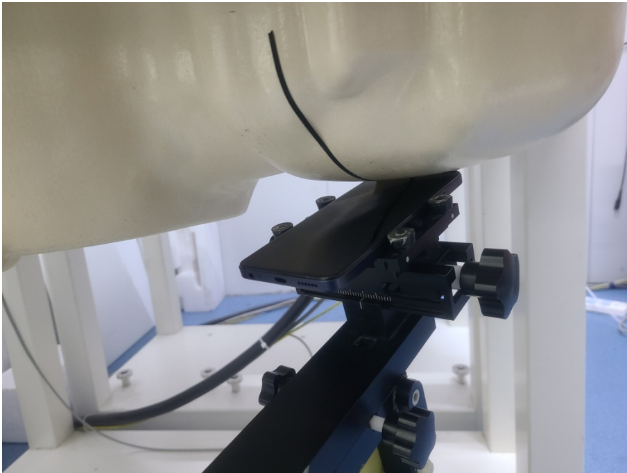
Head Left Tilt Setup Photo (0mm)
