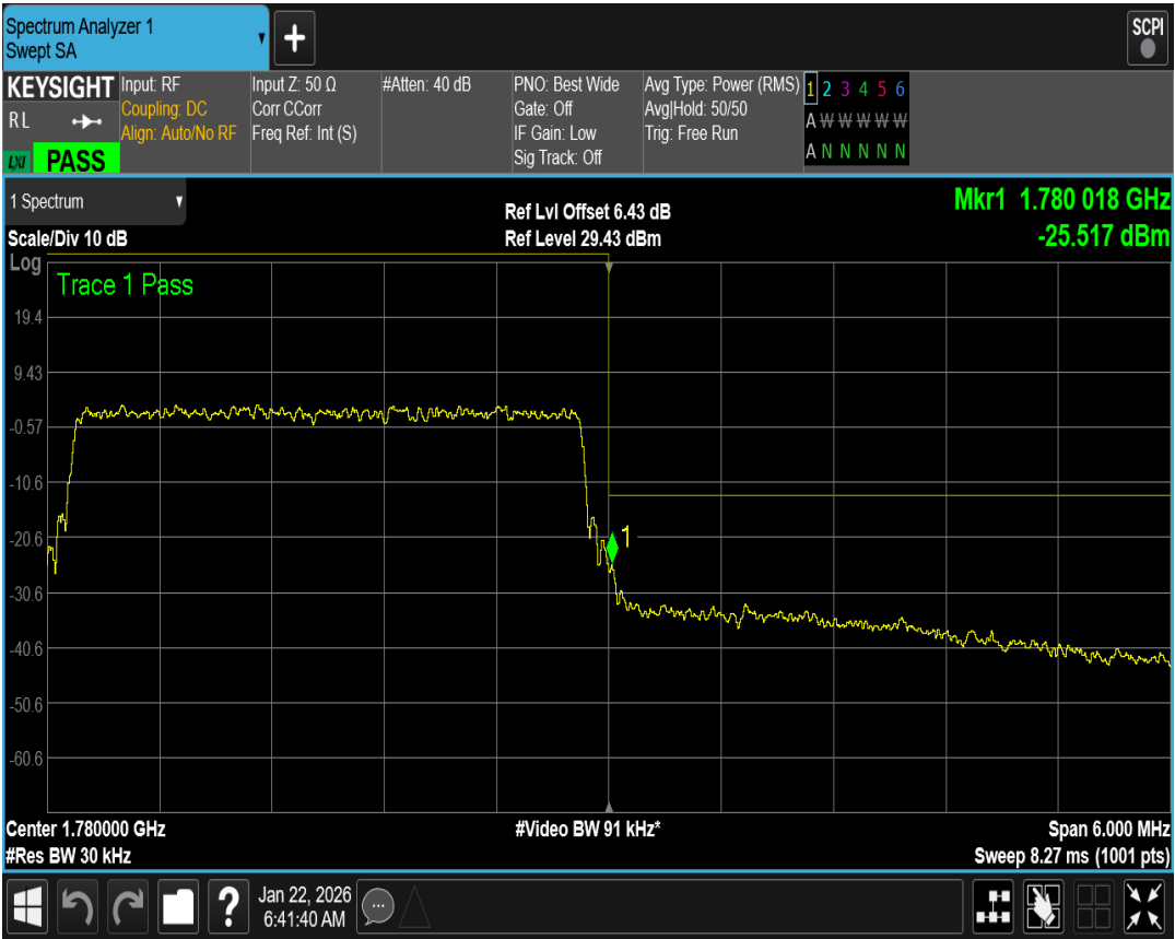
Band66 QPSK BW=1.4MHz Channel=132665 RB Size=6 Position=#0
