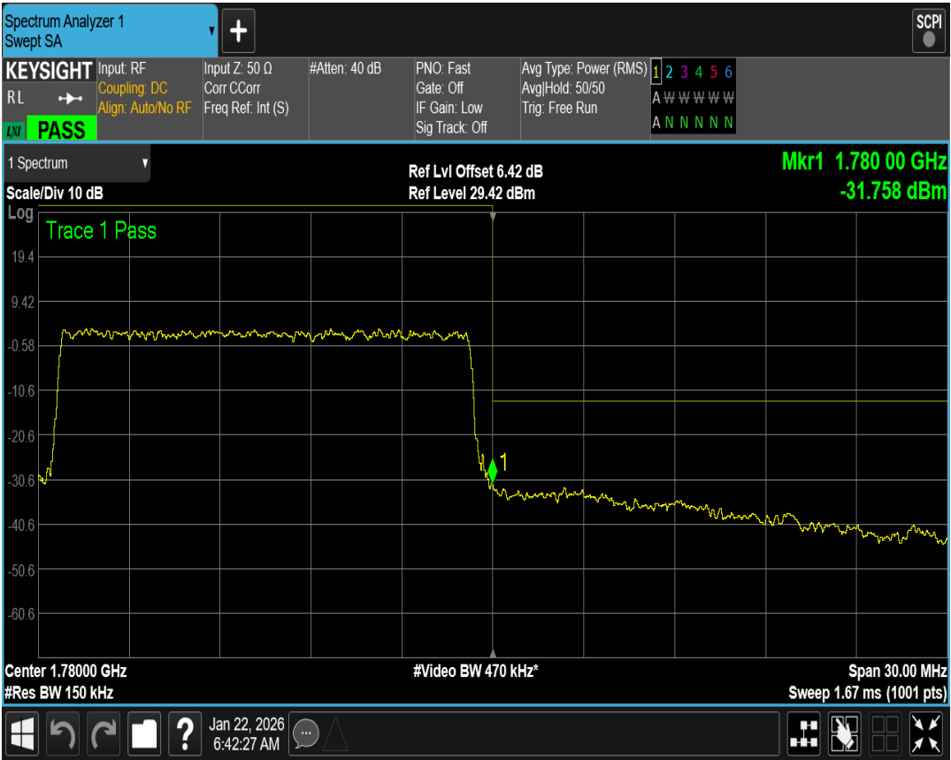
Band66 QAM16 BW=20MHz Channel=132072 RB Size=100 Position=#0
