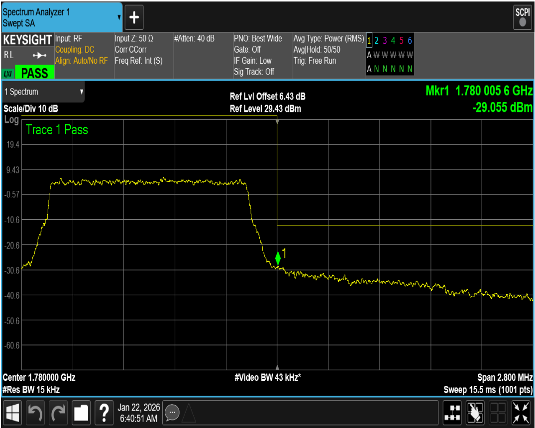
Band66 QPSK BW=10MHz Channel=132022 RB Size=50 Position=#0
