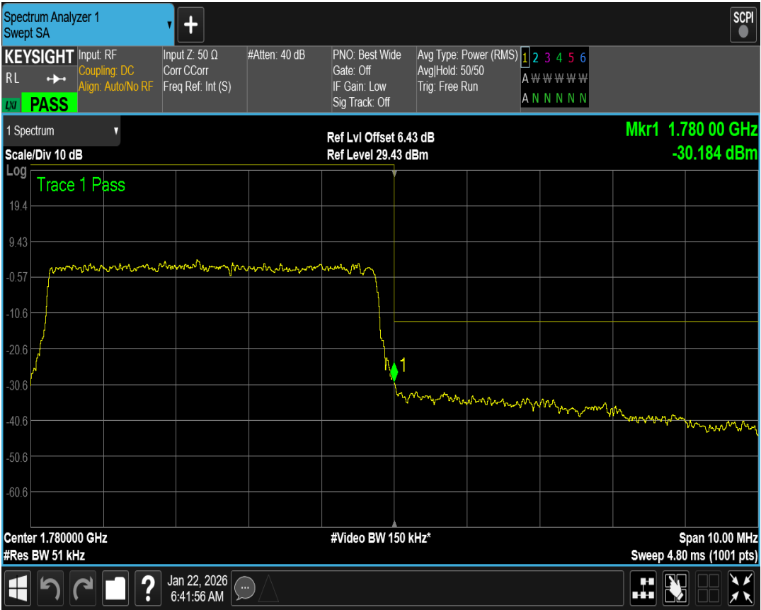
Band66 QPSK BW=1.4MHz Channel=131979 RB Size=6 Position=#0
