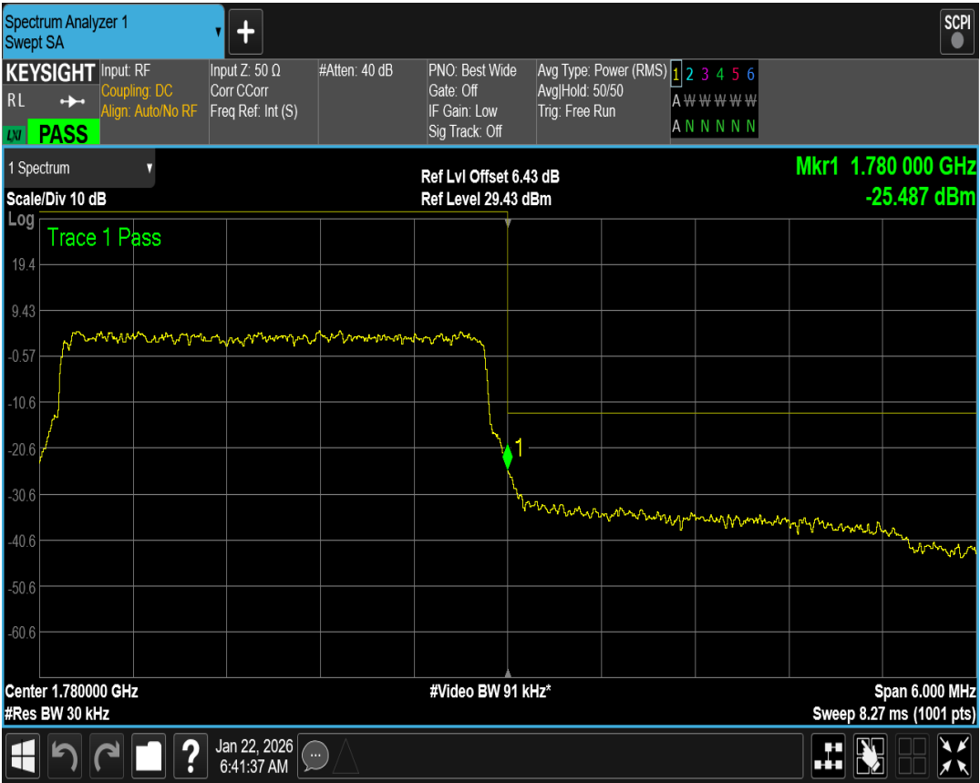
Band66 QPSK BW=5MHz Channel=131997 RB Size=25 Position=#0
