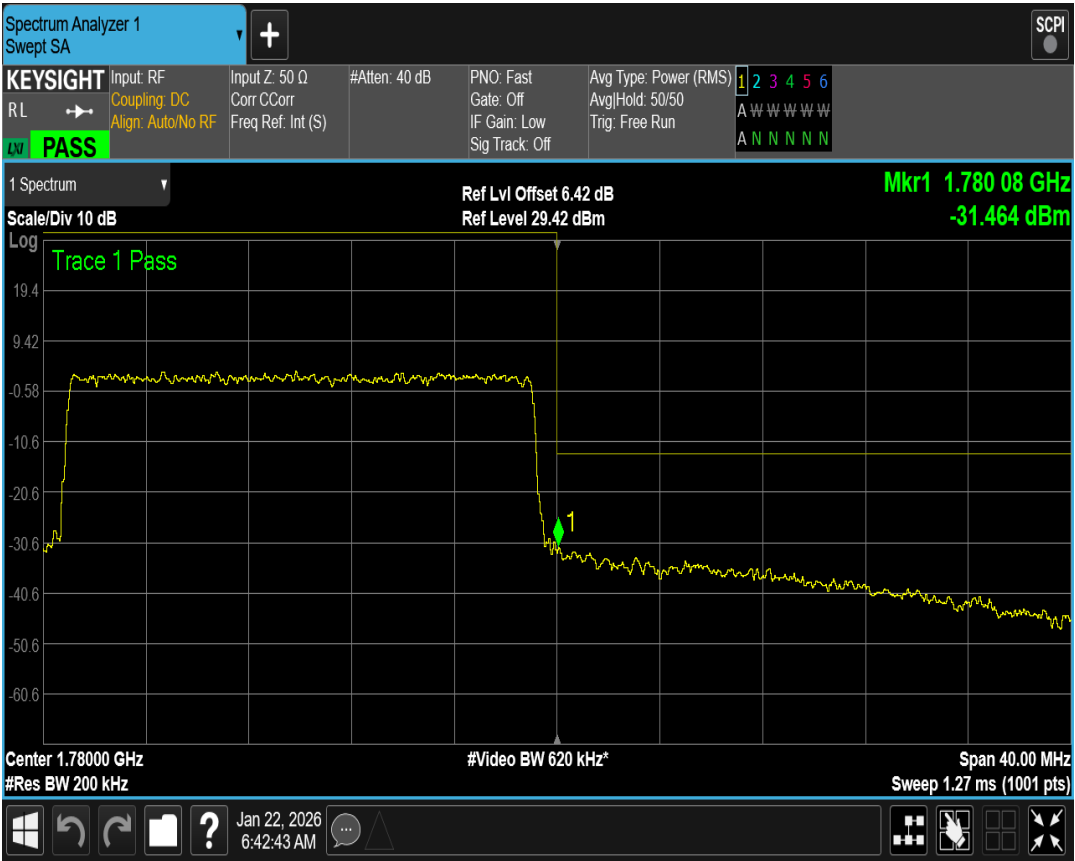
Band66 QAM16 BW=3MHz Channel=132657 RB Size=15 Position=#0
