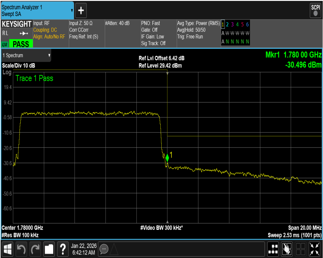
Band66 QAM16 BW=15MHz Channel=132047 RB Size=75 Position=#0
