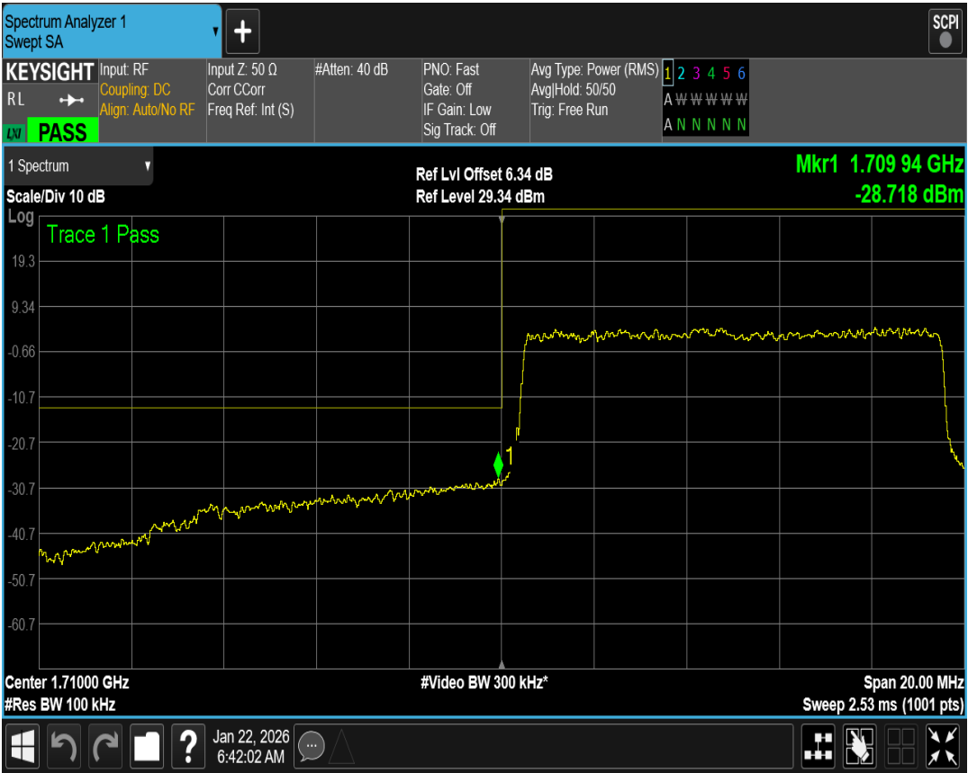
Band66 QPSK BW=10MHz Channel=132622 RB Size=50 Position=#0
