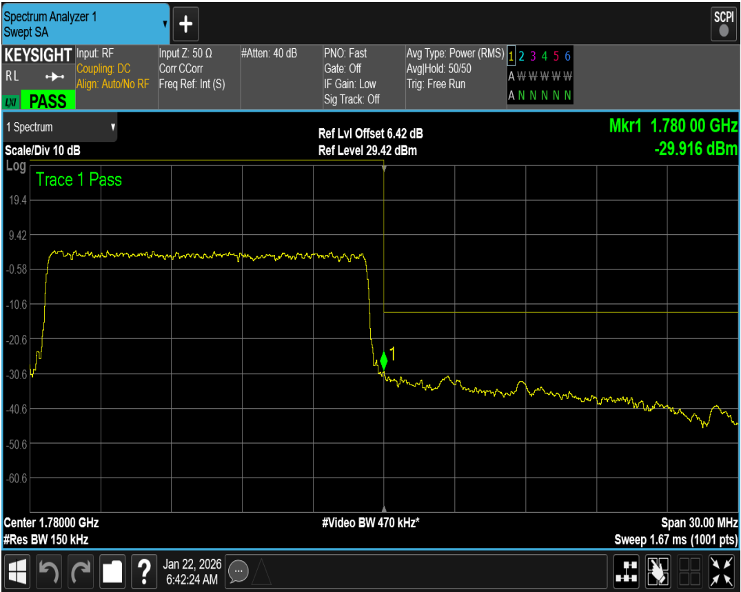
Band66 QPSK BW=20MHz Channel=132072 RB Size=100 Position=#0
