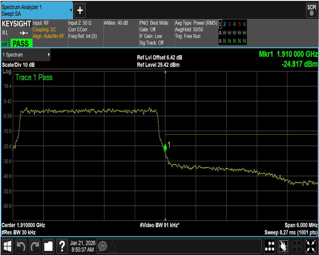
Band2 QPSK BW=5MHz Channel=18625 RB Size=25 Position=#0
