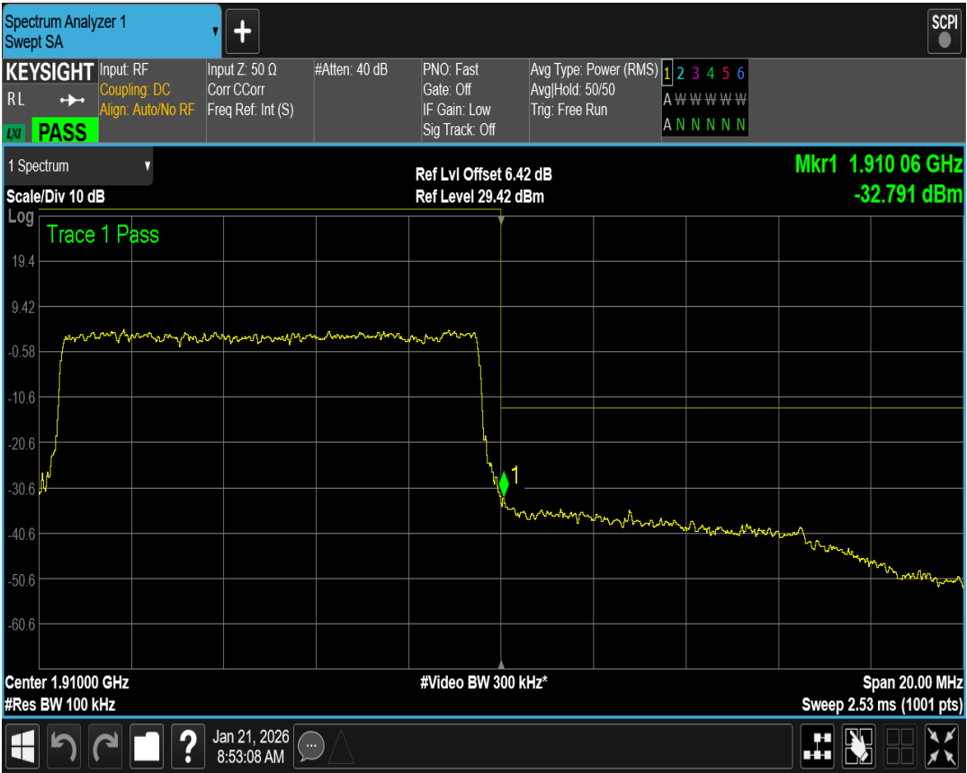
Band2 QPSK BW=1.4MHz Channel=18607 RB Size=6 Position=#0
