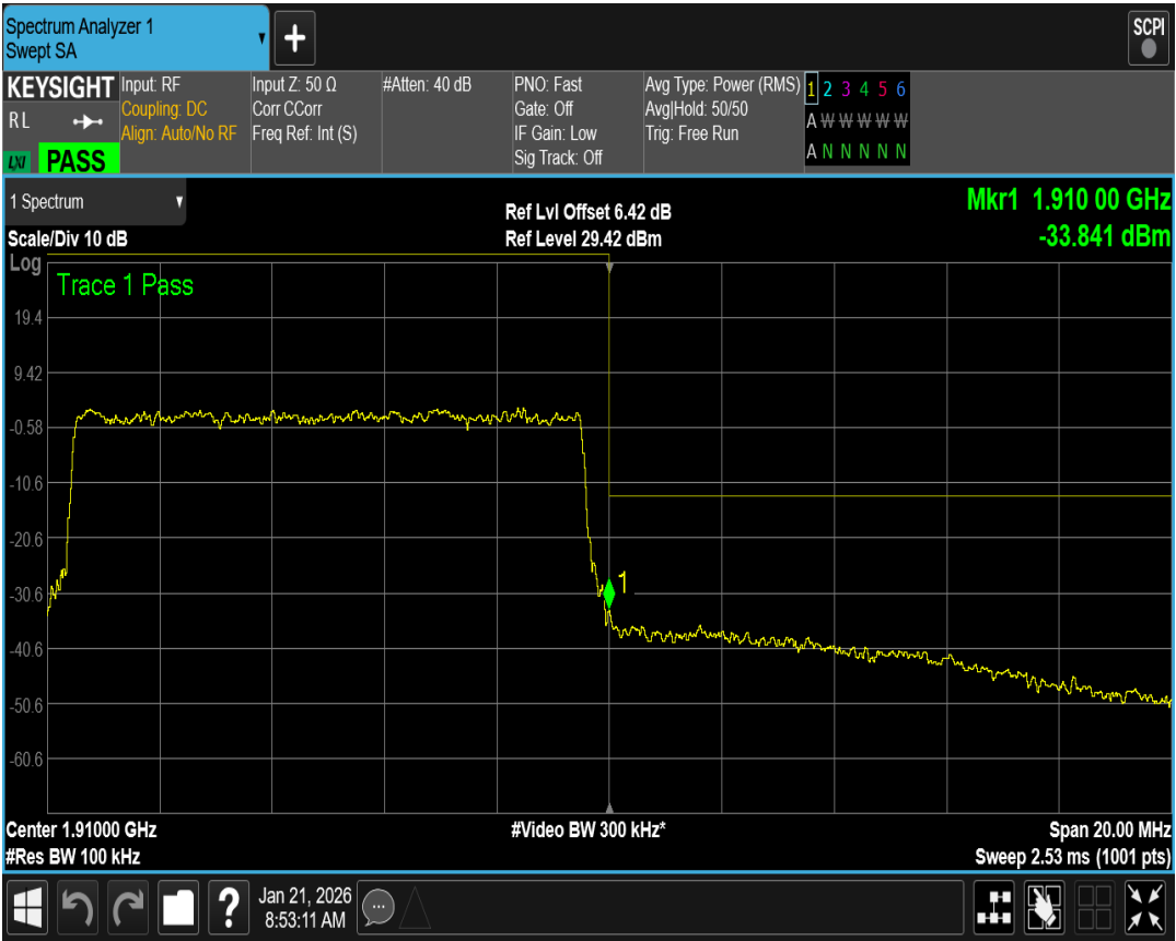
Band2 QAM16 BW=10MHz Channel=18650 RB Size=50 Position=#0
