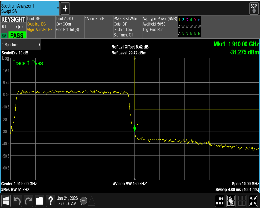
Band2 QAM16 BW=5MHz Channel=18625 RB Size=25 Position=#0
