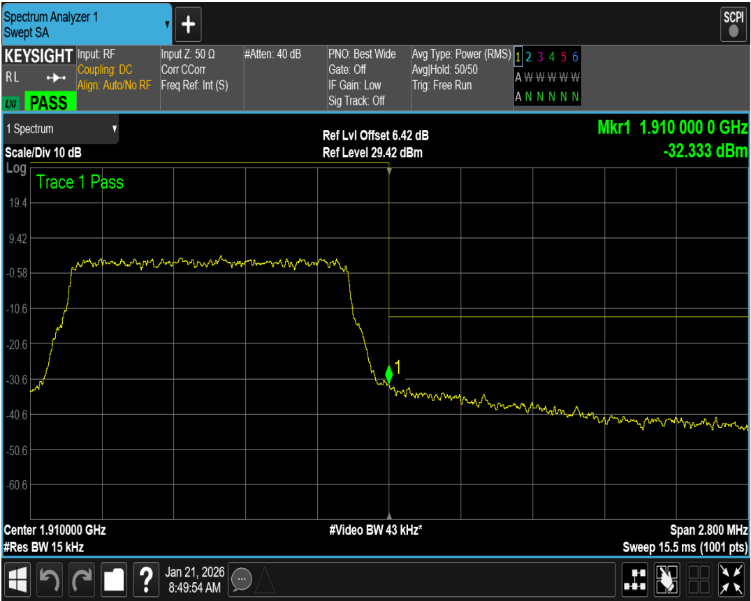
Band2 QAM16 BW=1.4MHz Channel=18607 RB Size=6 Position=#0
