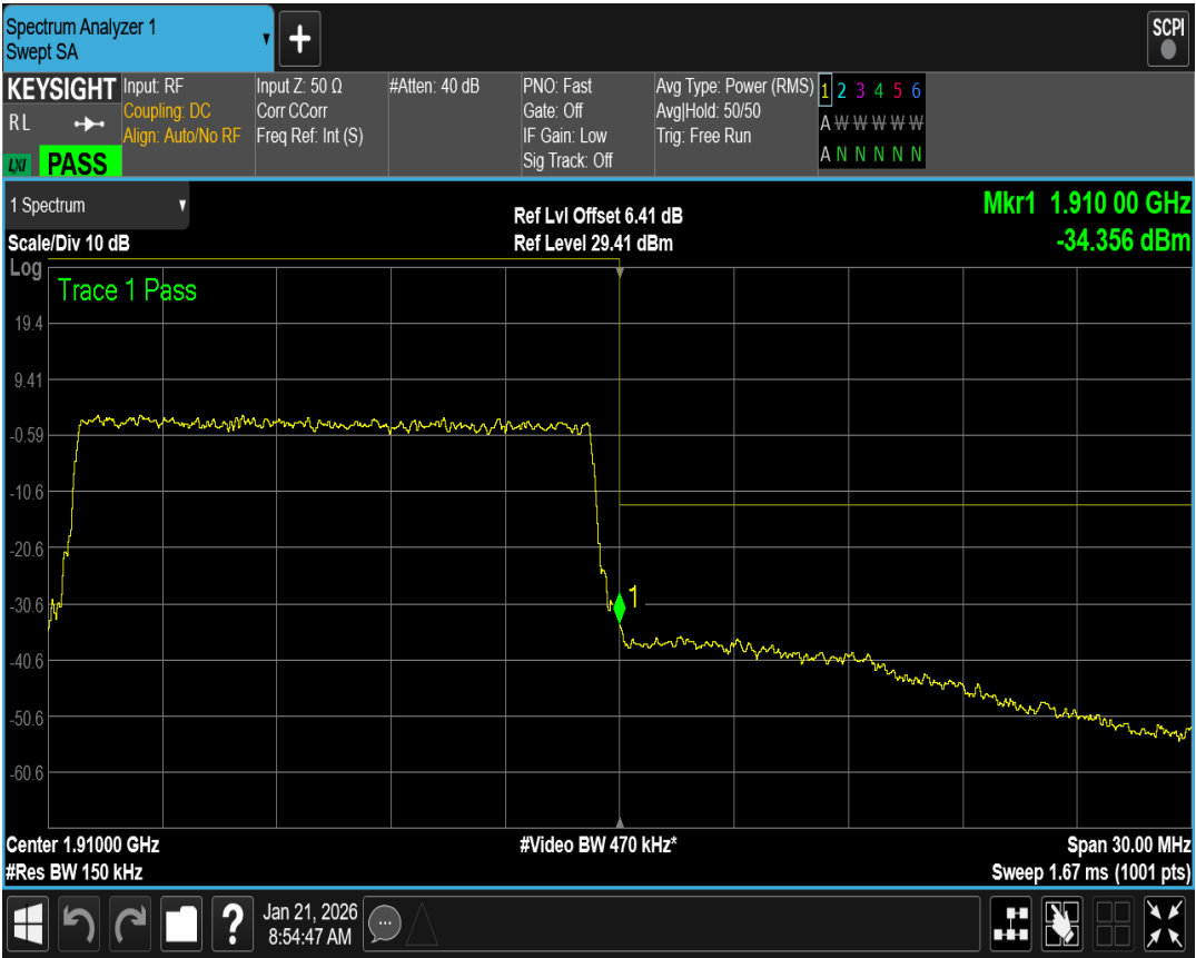
Band2 QAM16 BW=15MHz Channel=18675 RB Size=75 Position=#0
