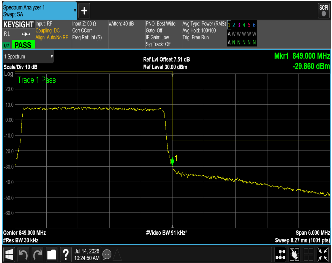
Band5 QAM16 BW=5MHz Channel=20425 RB Size=25 Position=#0
