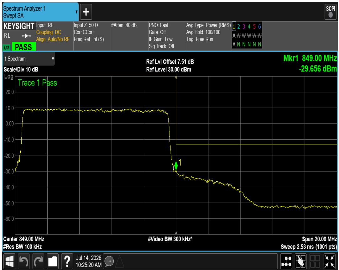
Band5 QPSK BW=3MHz Channel=20415 RB Size=15 Position=#0
