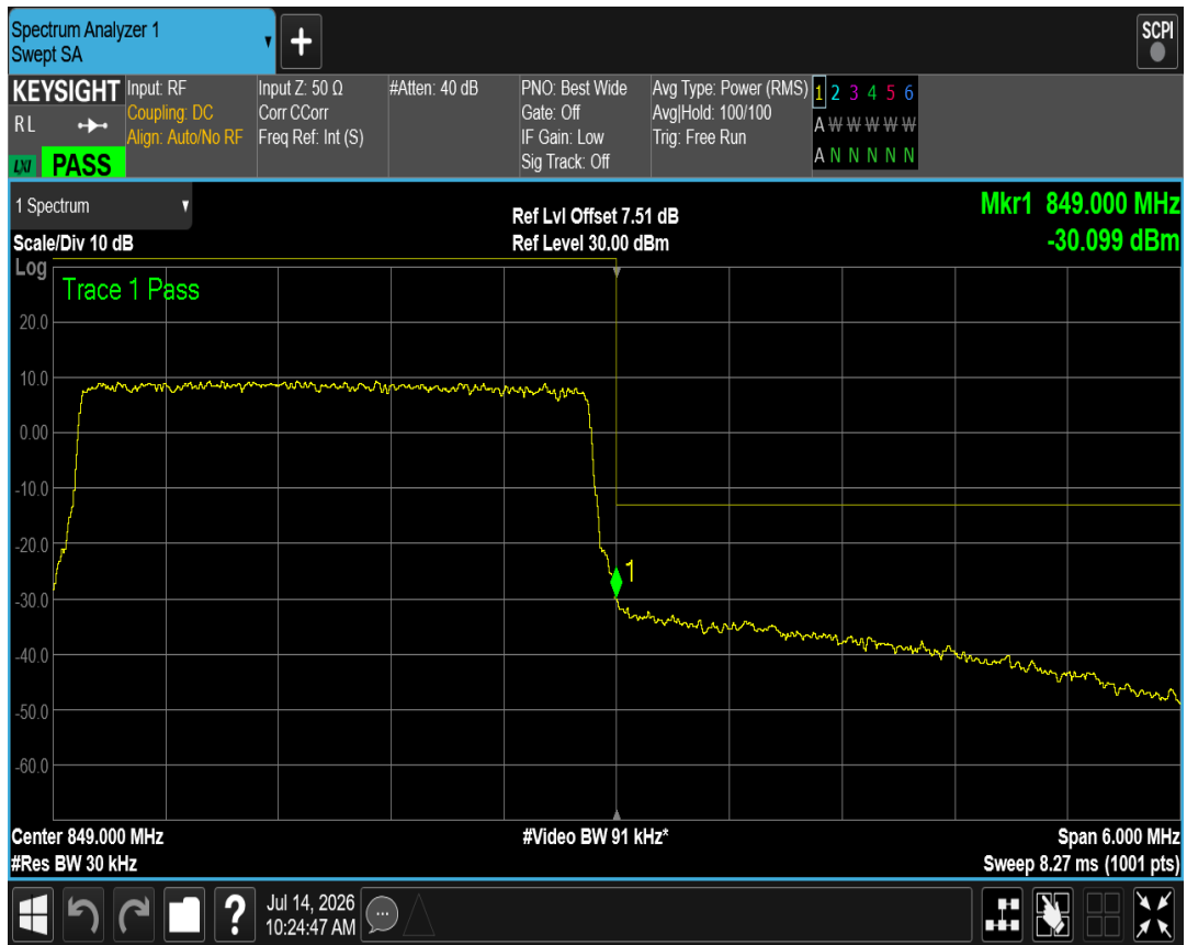
Band5 QPSK BW=5MHz Channel=20425 RB Size=25 Position=#0
