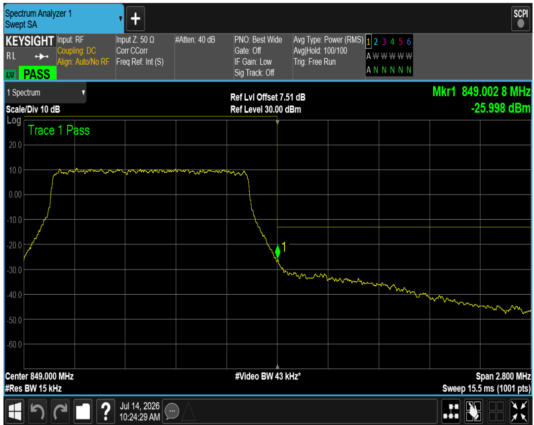
Band5 QPSK BW=10MHz Channel=20450 RB Size=50 Position=#0
