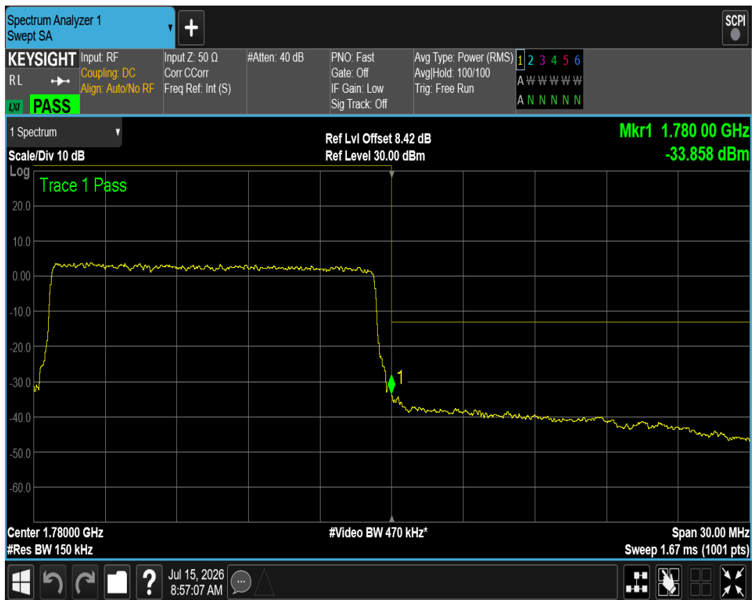
Band66 QAM16 BW=20MHz Channel=132072 RB Size=100 Position=#0
