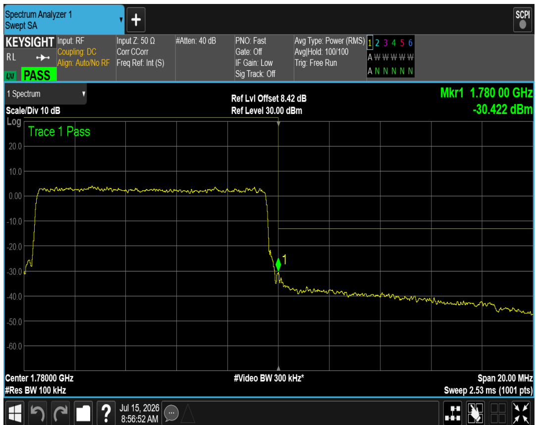
Band66 QAM16 BW=15MHz Channel=132047 RB Size=75 Position=#0
