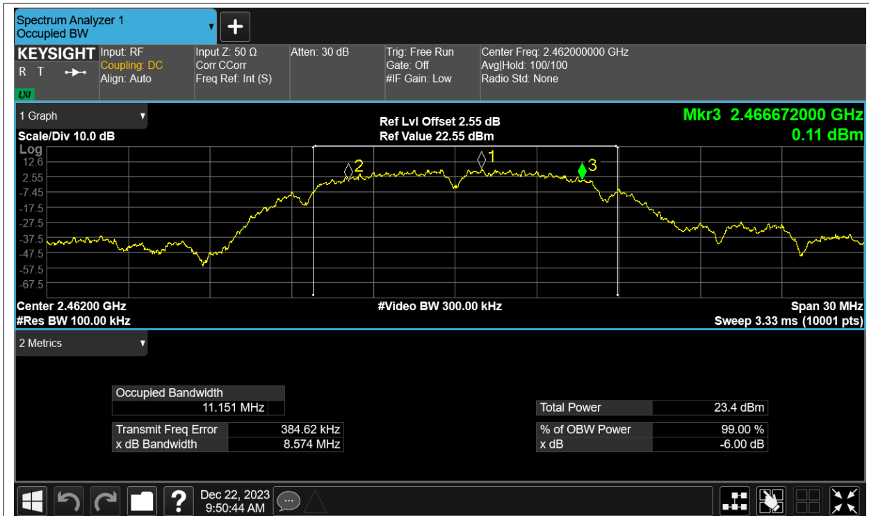
-6dB Bandwidth NVNT g 2412MHz Ant1
