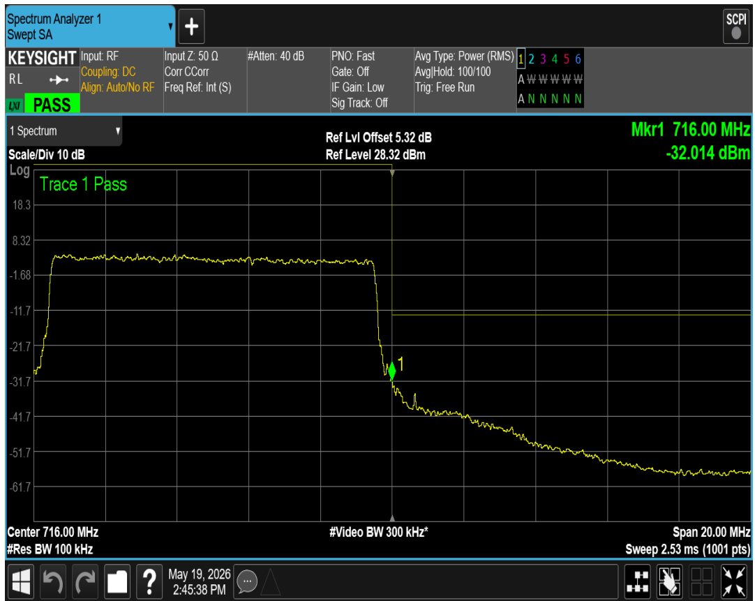
Band17 QPSK BW=5MHz Channel=23755 RB Size=25 Position=#0
