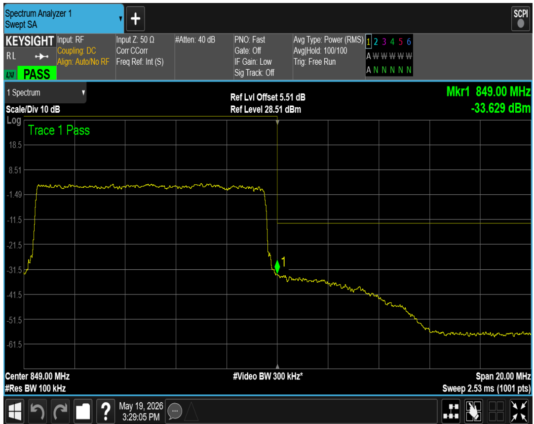
Band26(824-849) QAM16 BW=15MHz Channel=26865 RB Size=75 Position=#0
