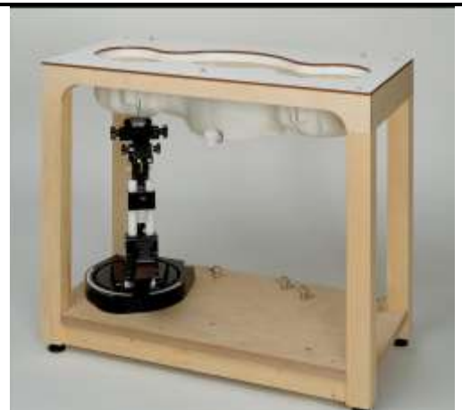
Fig. 8.7 Photo of SAM Twin Phantom
