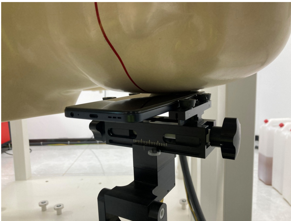
Head Left Cheek Setup Photo
