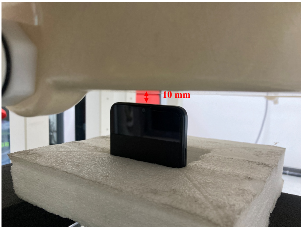
Body Top Setup Photo (10mm)
