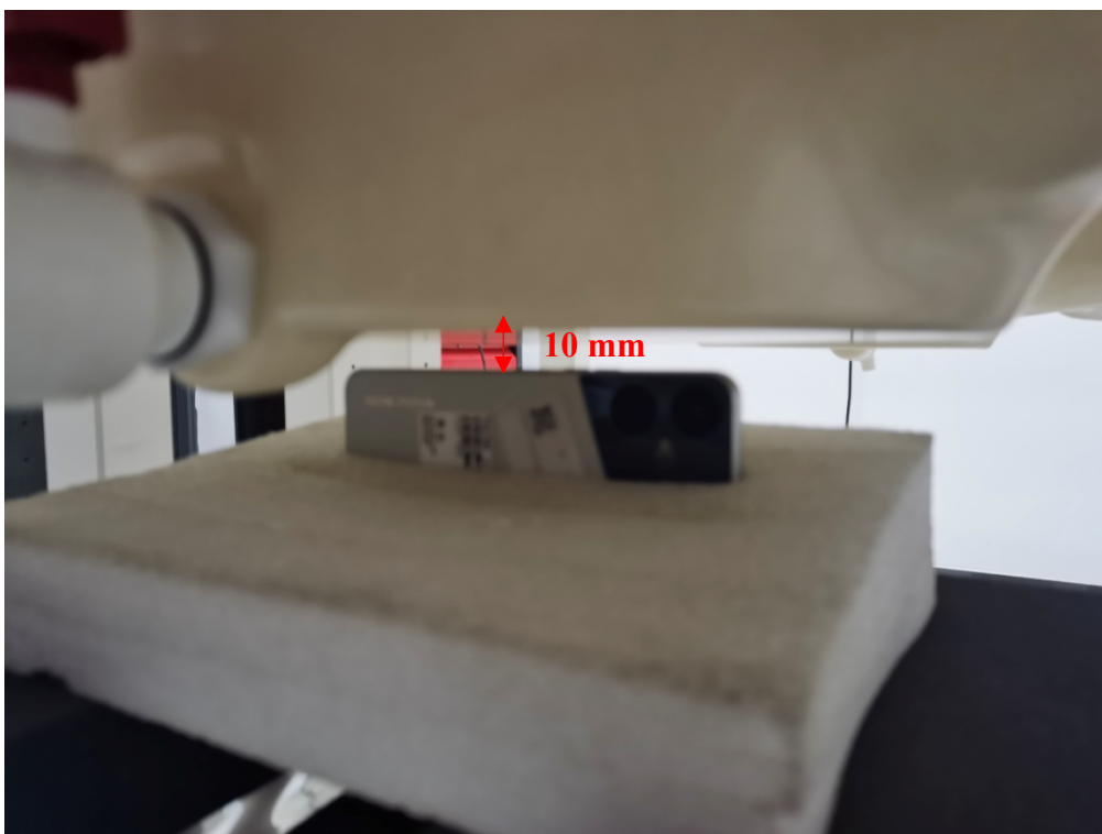
Body Right Setup Photo (10mm)
