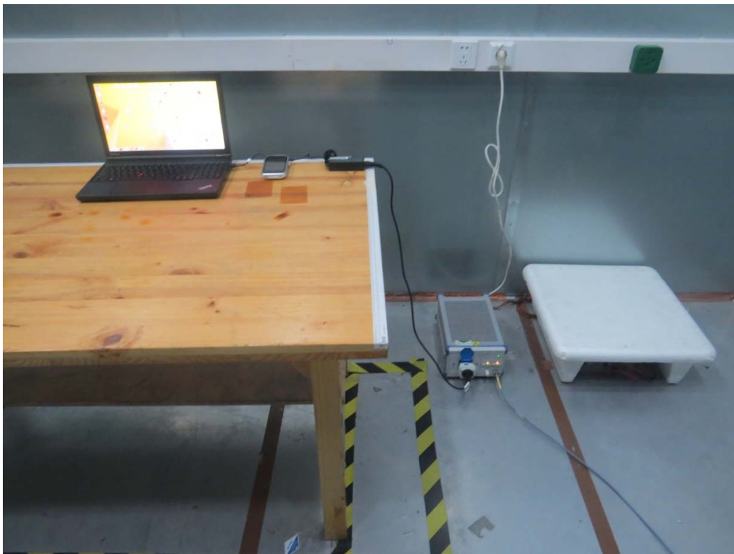
Picture 3 Conducted Emission Test Setup
