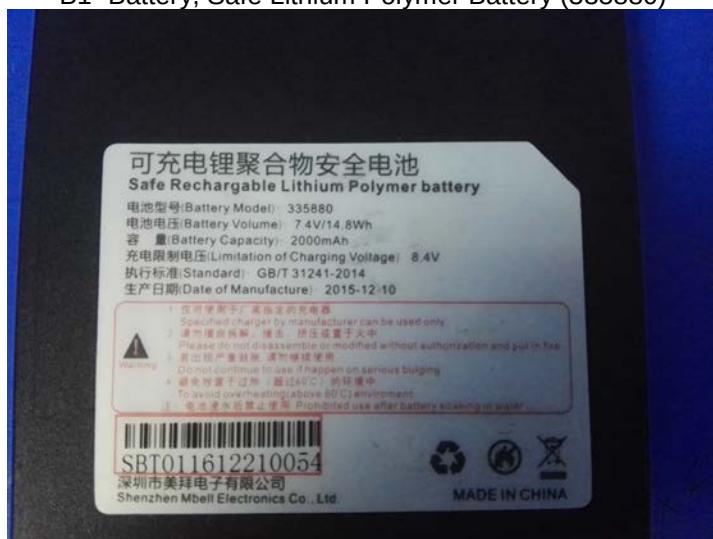
B1- Battery, Safe Lithium Polymer Battery (335880)
