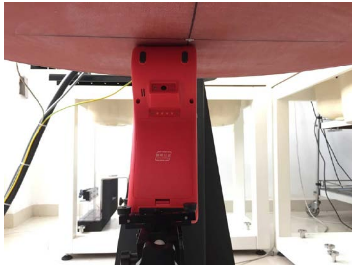
Handheld, the top of the EUT towards phantom (0mm)
