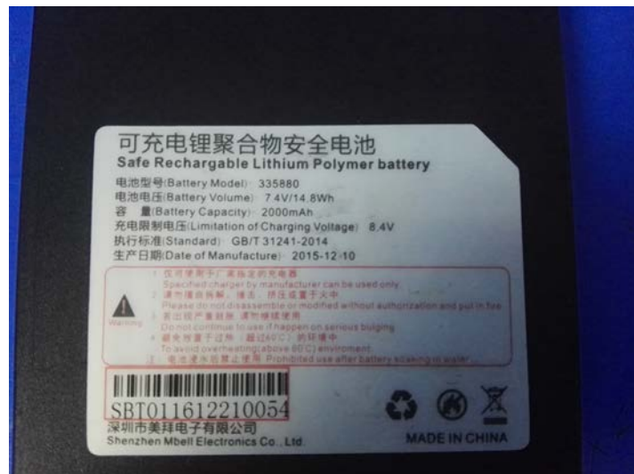
B1- Battery, Safe Lithium Polymer Battery (335880)
