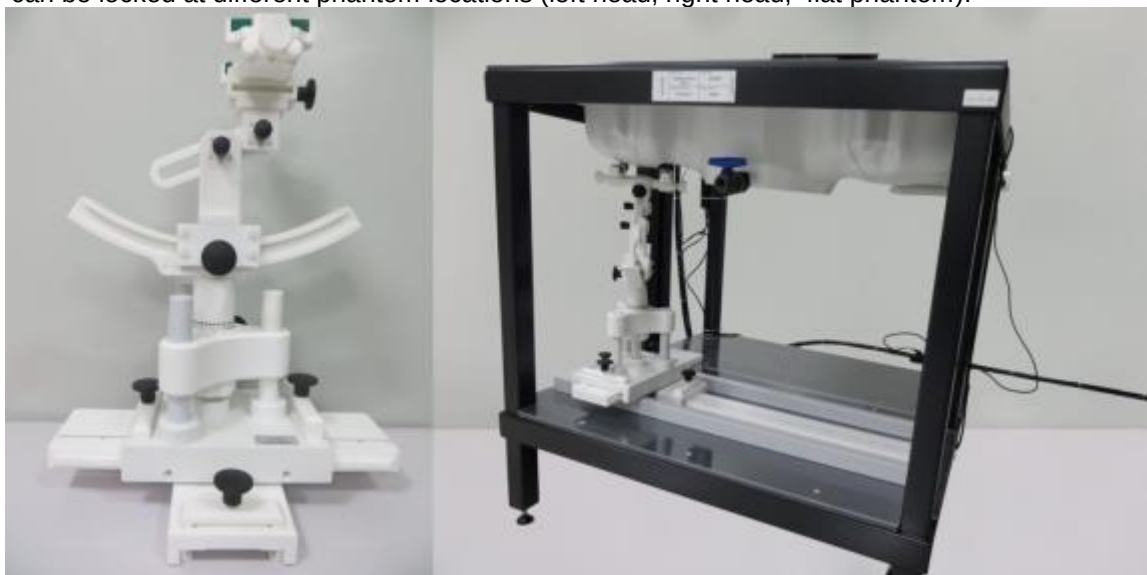
Device holder supplied by SATIMO
