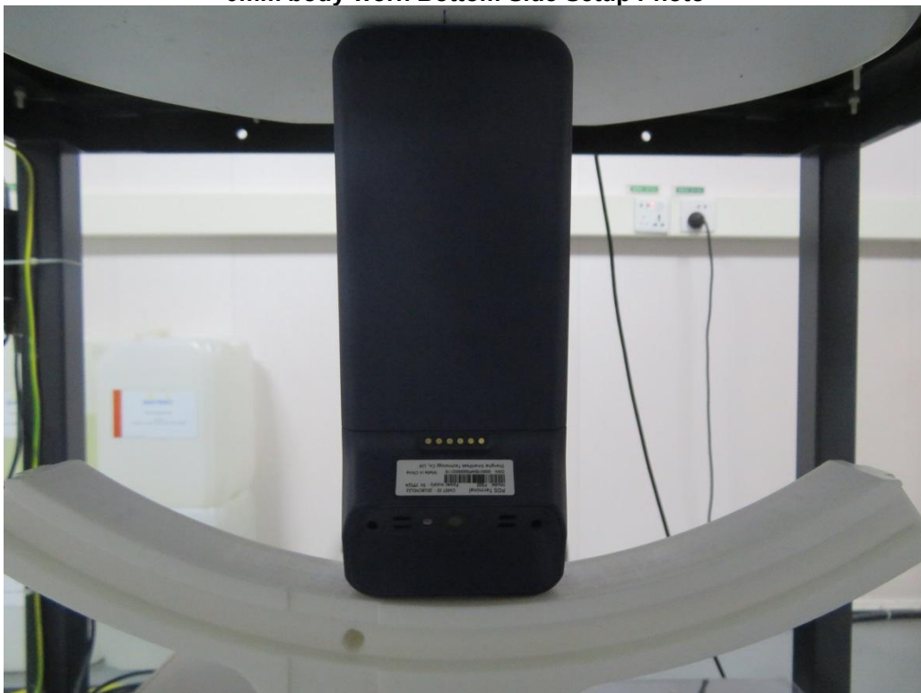
0mm body-worn Bottom Side Setup Photo
