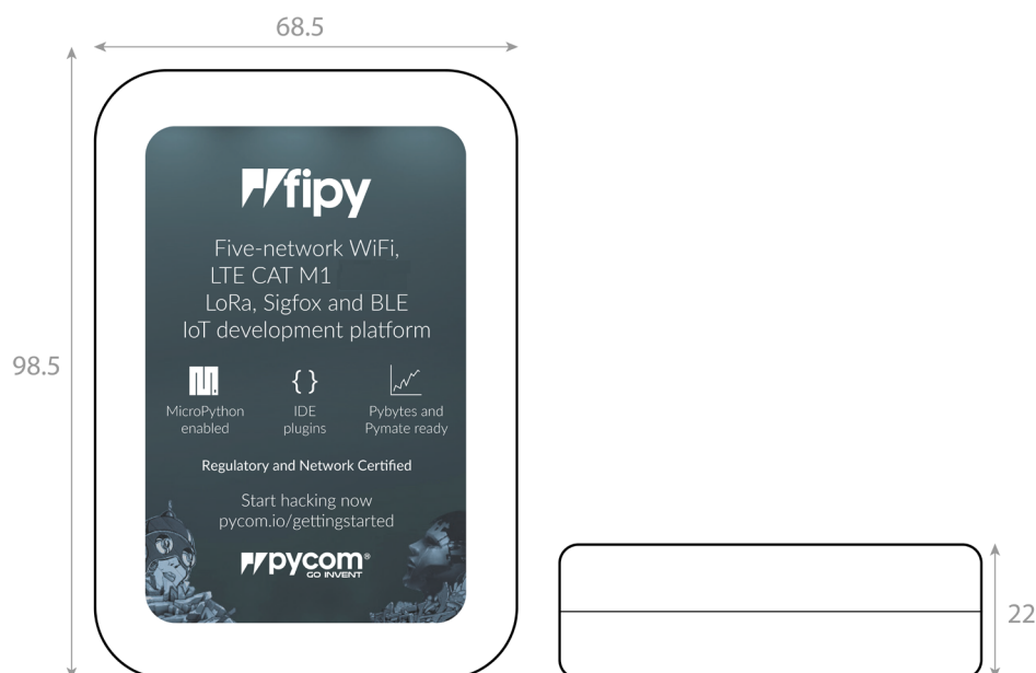
Figure 7 – Mechanical drawing of packaging – Units: mm
