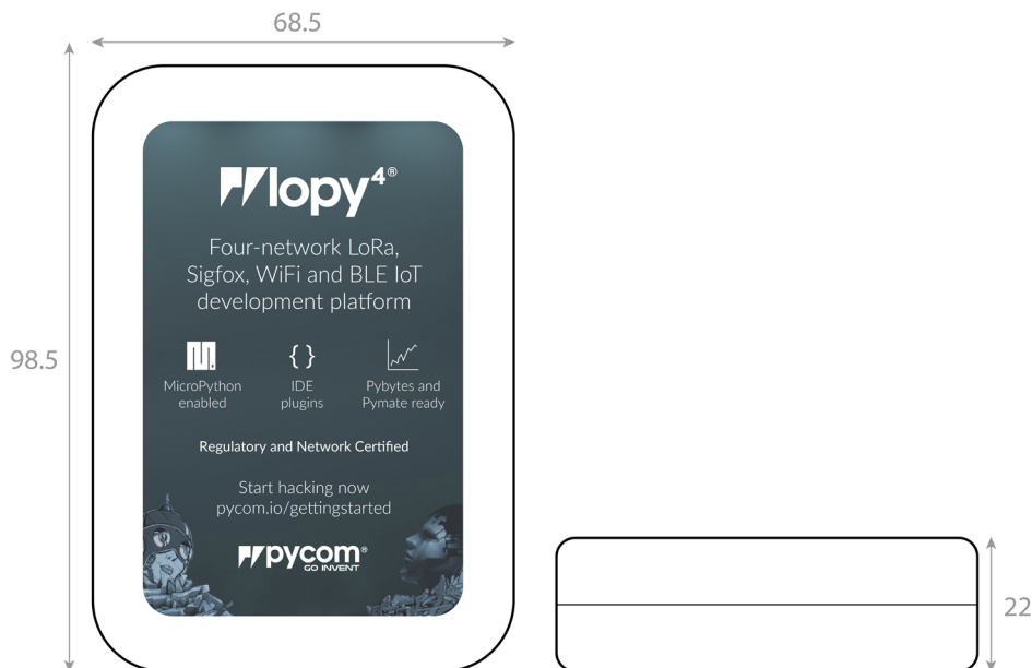
Figure 10 – Mechanical drawing of packaging – Units: mm
