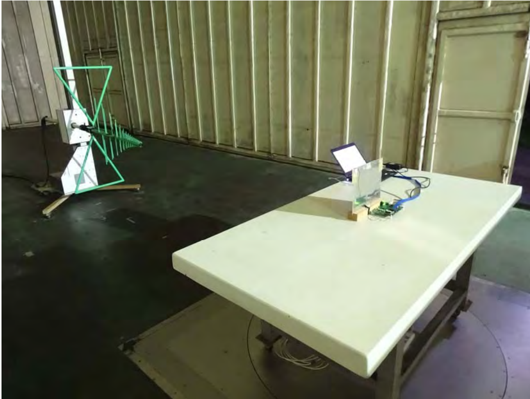
Front View of Radiated Test
