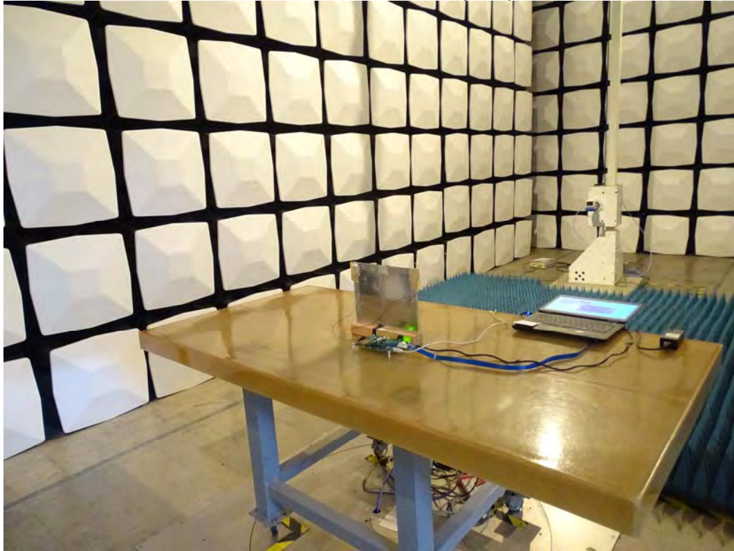
Back View of Radiated Test (Horn)
