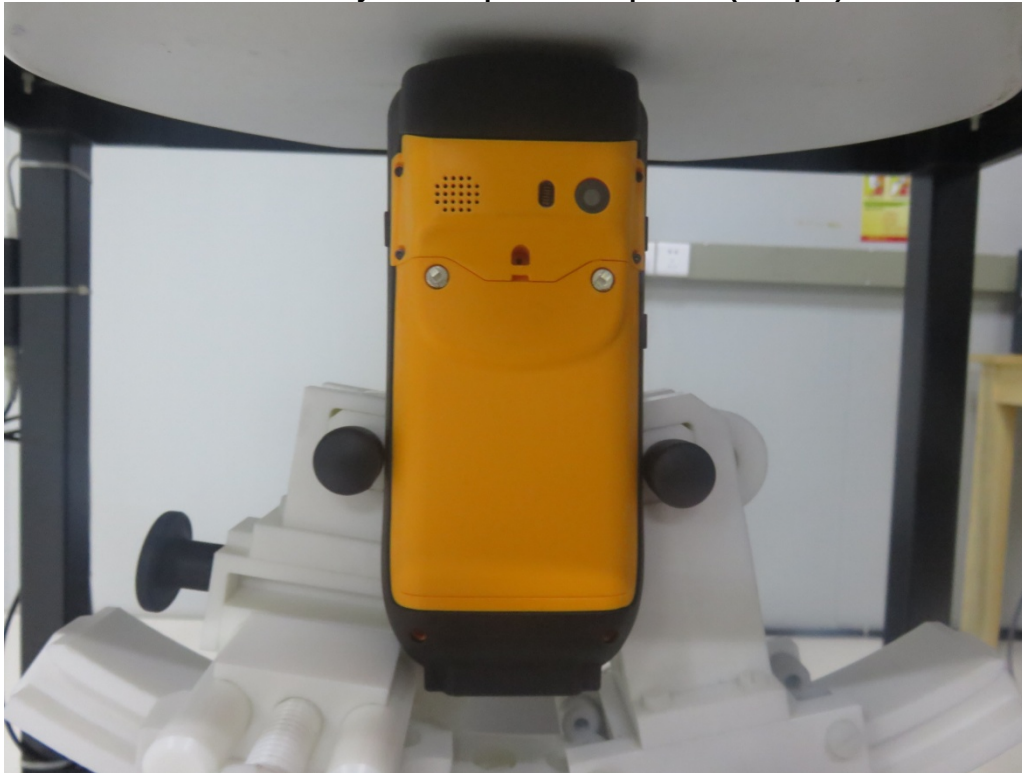
0mm body-worn Top Side Setup Photo(hotspot)
