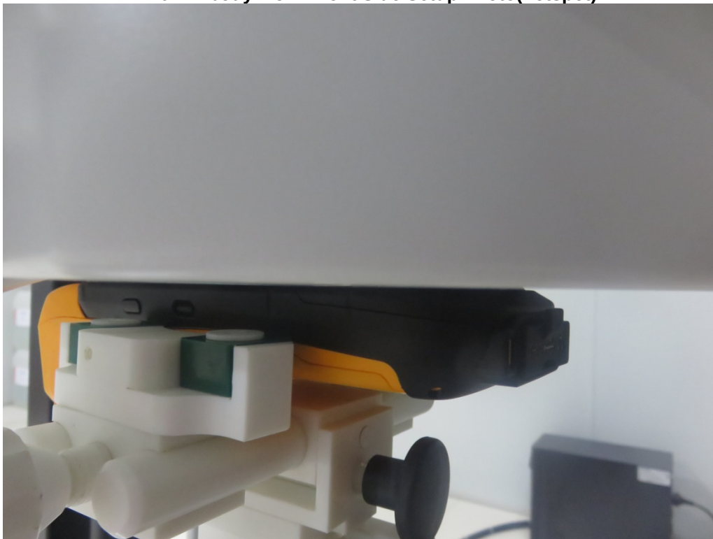
0mm body-worn Front Side Setup Photo(hotspot)
