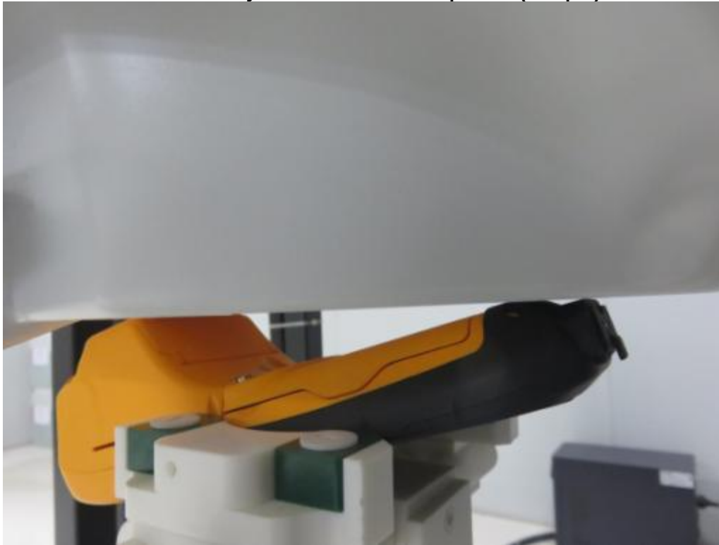
0mm body-worn Back Side Setup Photo(hotspot)
