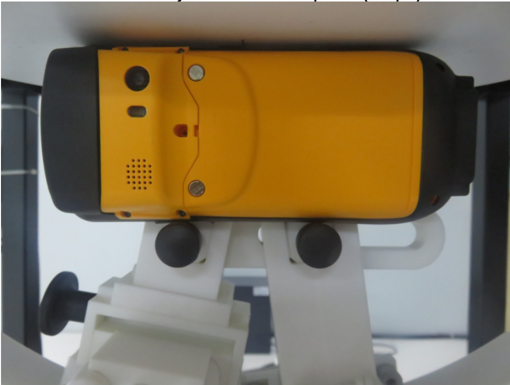
0mm body-worn Left Side Setup Photo(hotspot)
