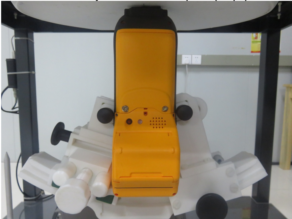
0mm body-worn Bottom Side Setup Photo(hotspot)
