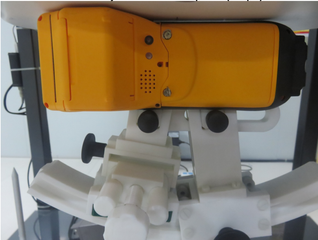
0mm body-worn Left Side Setup Photo(hotspot)
