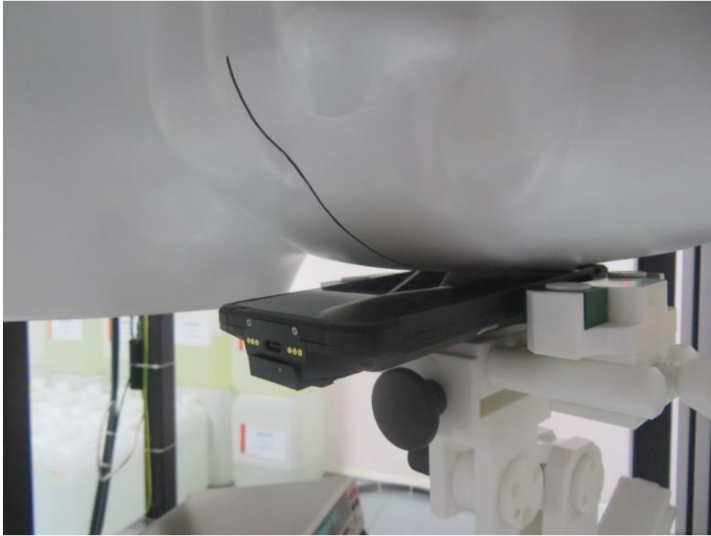
Head Setup Photo (Left Cheek)
